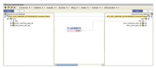
Note that the **IDOC\_INBOUND\_ASYNCRONOUS** is used to send and receive IDOCs via Transactional RFC (Asynchronous operation). Therefore, the Transaction Mode Configuration of the BAPI eWay in the Connectivity Map should always be set to "Transactional RFC" when using this OTD, as seen in Figure 93.
